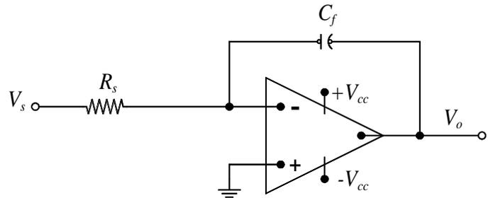
$$V_o = -\frac{1}{R_s C_f} \int_{t_0}^t V_s \, d\tau + V_o(t_0)$$
