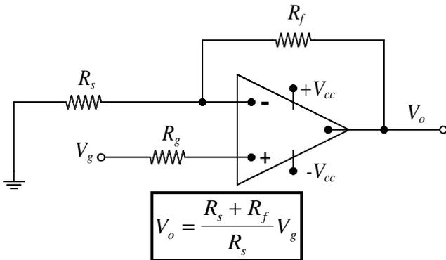
$$V_o = \frac{R_s + R_f}{R_s} V_g$$
