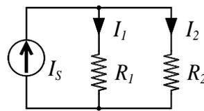
$$I_1 = \frac{R_2}{R_1 + R_2} I_s$$
