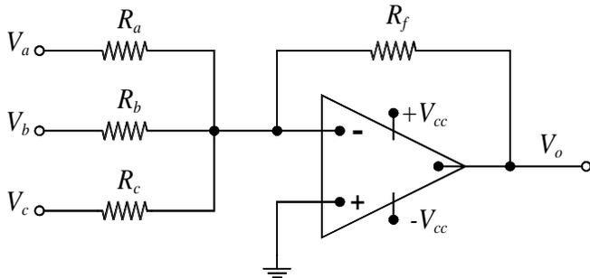
$$V_o = -\left(\frac{R_f}{R_a} V_a + \frac{R_f}{R_b} V_b + \frac{R_f}{R_c} V_c\right)$$
