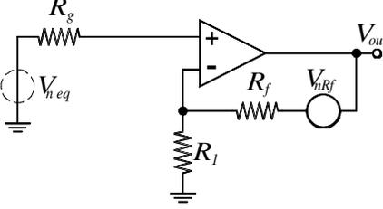
In this case, the noise at the output due to  $V_{nRf}$  is simply  $V_{nRf}$ .
