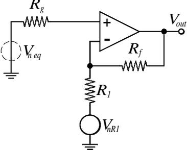
Under asymptotic conditions, the negative input of the op amp is at ground potential and no current enters the op amp, so all of the current generated by  $V_{nR1}$  (which is  $V_{nR1}/R_1$ ) goes through  $R_f$  to create a voltage at the output ( $-V_{nR1}R_f/R_1$ ).
