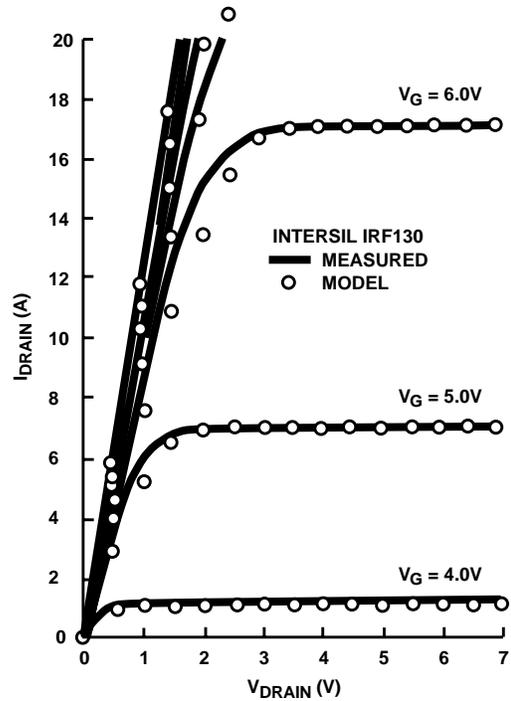
FIGURE 8. PLOTS OF DRAIN CURRENT vs. DRAIN VOLTAGE FOR THE INTERSIL IRF130 POWER MOSFET SHOW AN EXCELLENT FIT BETWEEN MEASURED VALUES AND THOSE CALCULATED BY THE ENHANCED SPICE II MODEL FOR VARIOUS VALUES OF CONSTANT GATE VOLTAGE.
