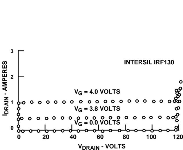
FIGURE 9. FIRST QUADRANT DRAIN CURRENT vs. DRAIN VOLTAGE WITH  $V_{GS}$  HELD CONSTANT IS CALCULATED BY THE ENHANCED SPICE II MODEL OF THE INTERSIL IRF130 POWER MOSFET. NOTE THAT THE MODEL PREDICTS AVALANCHE BREAKDOWN.
