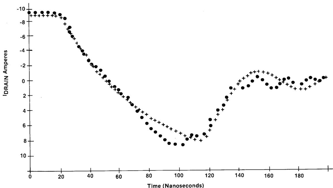
FIGURE 13. THE CALCULATED THIRD-QUADRANT DIODE RECOVERY WAVEFORM OF THE ENHANCE SPICE II MODEL SHOWS GOOD AGREEMENT WITH THAT ACTUALLY MEASURED FOR THE INTERSIL IRF130 POWER MOSFET
