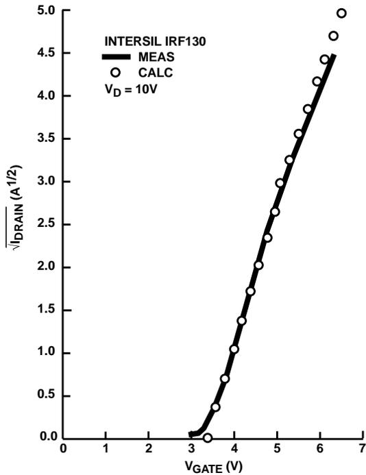
FIGURE 7. MEASURED SQUARE ROOT OF DRAIN CURRENT (DRAIN VOLTS = 10) vs. GATE VOLTAGE FOR THE INTERSIL IRF130 POWER MOSFET IS PLOTTED ALONG WITH THE CALCULATED VALUES FOR THE ENHANCED SPICE II MODEL. AN EXCELLENT FIT IS OBTAINED.
