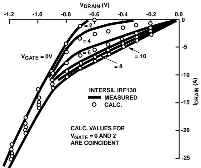
FIGURE 10. THIRD-QUADRANT OPERATION OF THE INTERSIL IRF130 SHOWS AGREEMENT BETWEEN THE PREDICTED VALUES OF THE ENHANCED SPICE II MODEL AND ACTUAL MEASURED VALUED OF DRAIN CURRENT vs DRAIN VOLTAGE AT DIFFERENT VALUED OF CONSTANT GATE VOLTAGE.
