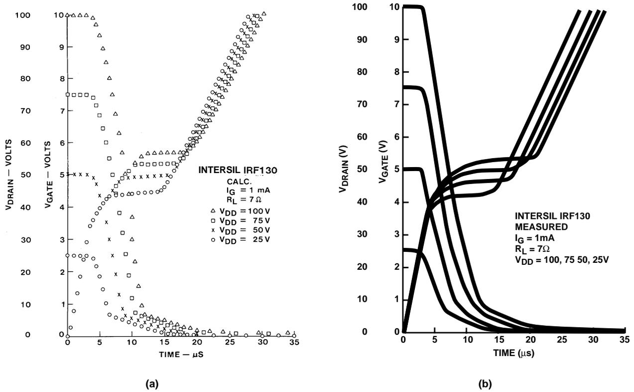
FIGURE 11. THESE PLOTS OF DRAIN AND GATE VOLTAGES vs. TIME FOR CONSTANT GATE CURRENT SHOW AGREEMENT BETWEEN THE PREDICTIONS OF THE ENHANCED SPICE II MODEL (a) AND MEASURED PERFORMANCE OF THE INTERSIL IRF130 POWER MOSFET (b).
