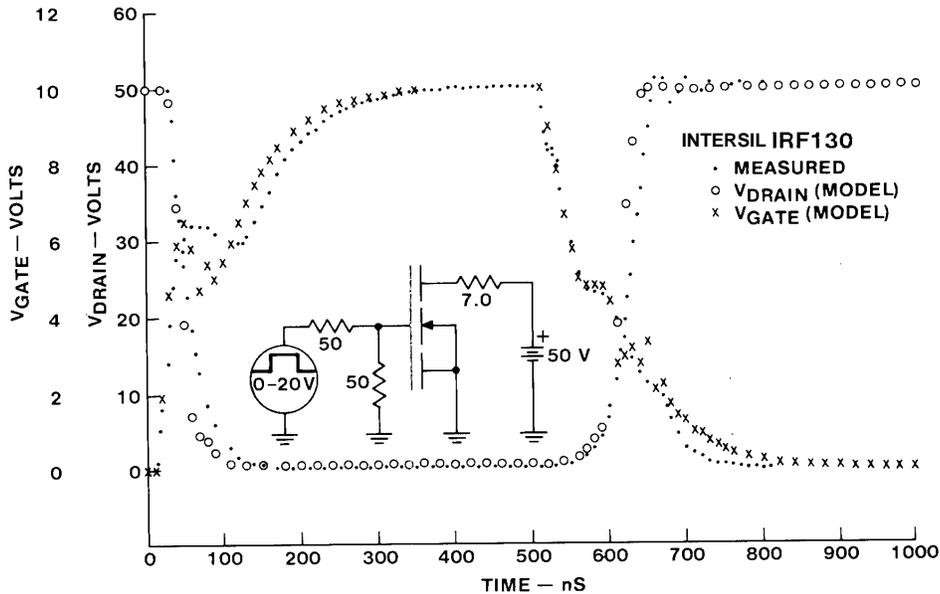
FIGURE 12. SWITCHING PERFORMANCE OF THE INTERSIL IRF130 POWER MOSFET IS CLOSELY PREDICTED BY THE ENHANCED SPICE II MODEL IN THIS PLOT OF MEASURED AND CALCULATED VALUES OF DRAIN AND GATE VOLTAGES vs. TIME IN A STANDARD SWITCHING CIRCUIT.
