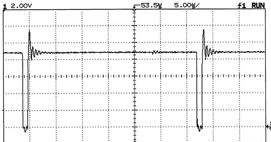
**30KHz square wave oscillator output**
