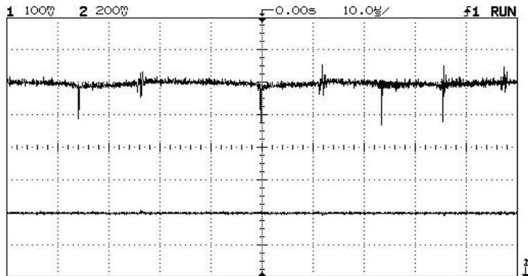
Input voltage (upper trace) and output voltage (lower trace) after adding the 820  $\mu\text{H}$  inductor and 470  $\mu\text{F}$  capacitor at the output. Output noise, which is on the 100  $\text{mV}$  per division scale (the smallest scale available on this equipment for a 25-volt signal), is barely perceptible, less than 10  $\text{mV}_{\text{pp}}$ , which is less than the 20  $\text{mV}$  maximum specification.
