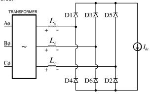
Consider the commutation interval between D5 and D1, when D1 has come on and D5 has not yet gone off. At this time D1, D5, and D6 are on and the other diodes are off. So the circuit looks like this:
