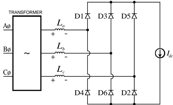
Consider the commutation interval between D5 and D1, when D1 has come on and D5 has not yet gone off. At this time D1, D5, and D6 are on and the other diodes are off. So the circuit looks like this:
