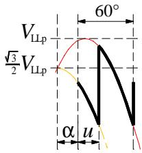
$$V_{dc} = \frac{1}{\pi/3} \left[ \int_{\alpha}^{\alpha+u} \frac{\sqrt{3}}{2} V_{LLP} \cos \theta d\theta + \int_{\alpha+u-\frac{\pi}{6}}^{\alpha+\frac{\pi}{6}} V_{LLP} \cos \theta d\theta \right]$$
