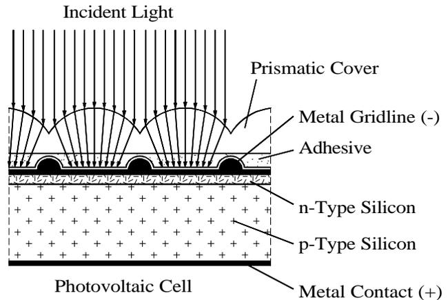
**Figure 3. Prism cover for high-current solar cell [12].**
