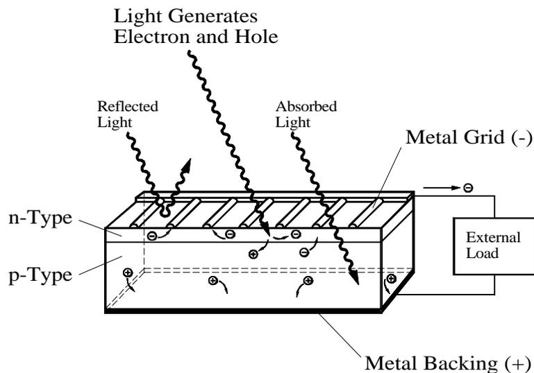
**Figure 1. How solar cells work [4, p. 22].**
